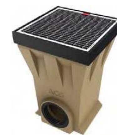
Gully made of polymer concrete with mesh grating Maschenrost (galvanized steel MW 32x10 mm) cast iron frame
